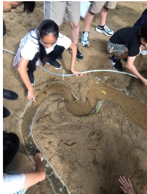
They observe erosion and sedimentation at the turns of their river models.
